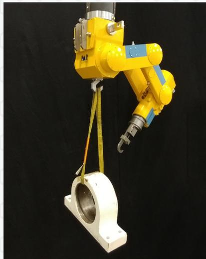
**High Capacity Lifting Hook**
