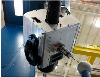
In order to maximize fidelity between the different process tools, they are all integrated into a single head. Two laser profilometers, the waterjet cutting head with its interchangeable catchers, and spindle with automatic tool change are mounted orthogonal to each other to prevent interference from one process in another process.
